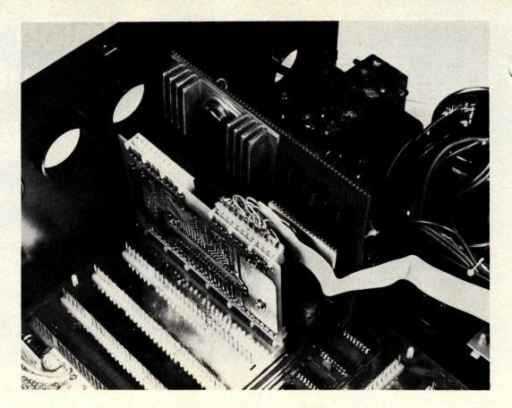
Photo 1: The multiplier installed in 10 slot 7 of the SwTPC 6800 processor system. The multiplier was constructed on a perforated board base, and is seen here between a parallel interface board and the power supply transformer. The heat sink for the multiplier's on board regulator tends to dominate the board, and the multiplier integrated circuit itself is the white 40 pin package partially hidden by a cable.
