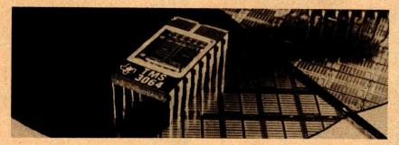
A new 64 K bit charge coupled device (CCD) memory has been announced by Texas Instruments. Designated the TMS3064, the memory is organized externally as 65,536 1 bit words and internally as 16 addressable 4096 bit serial-parallel-serial loops.
